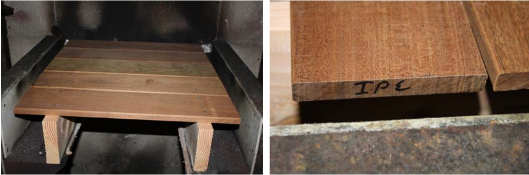
IPE prior to test
